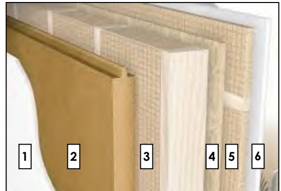
Structure from exterior to interior: 1-Plaster, 2-FD-Q11 protect , 3-Timber stud with holzFlex ® standard, 4-OSB board, 5-Battens with holzFlex ® standard, 6-Interior facing
