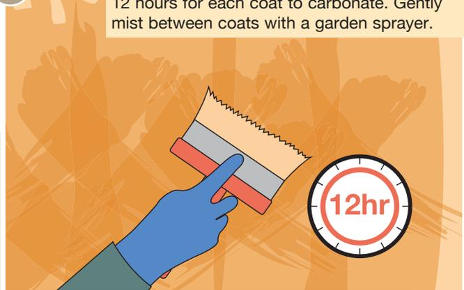
**Tip:** Internally: 3x coats minimum. Externally: 4x coats minimum. The thinner the coats, the better. Externally, 7 coats is not unusual if elevation is exposed!
